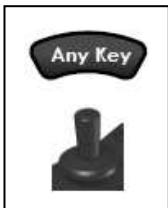
Press any button on the DX system or move the joystick. The DX system turns on.
