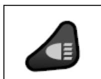
To turn the Headlights on, press the Headlight Button. The green Headlight LED next to button will lit. Press the Headlight Button again to turn the headlights off.
